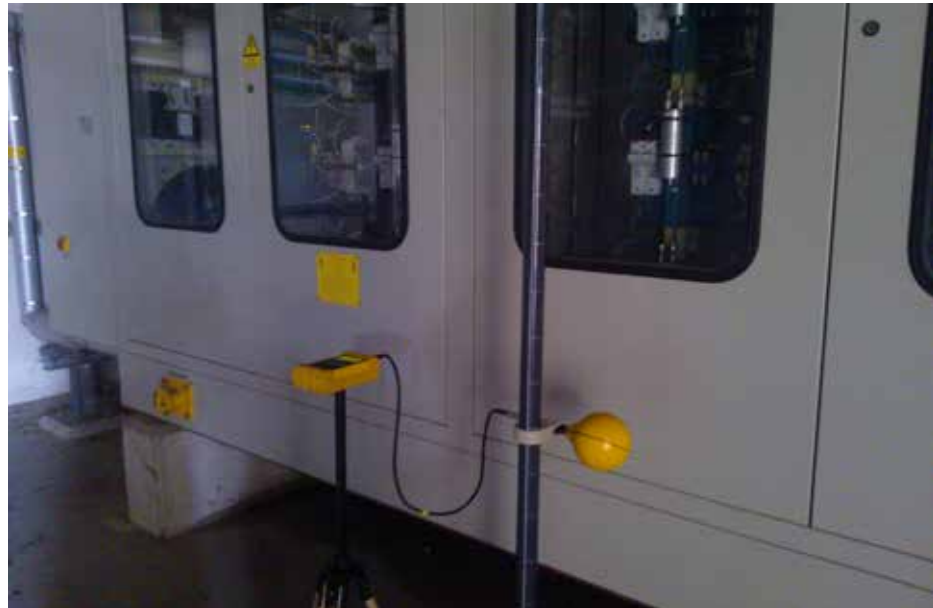
Figure 3.6 — Measurements being made near a thyristor rectifier
